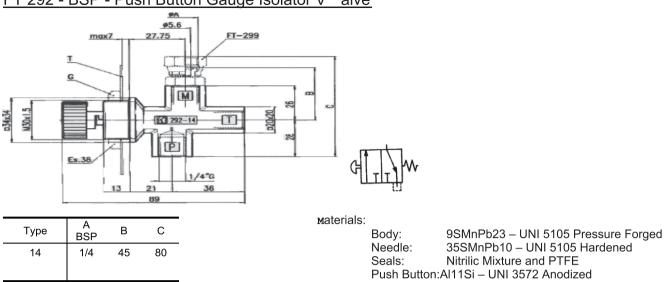
FT 292 - BSP - Push Button Gauge Isolator V alve
