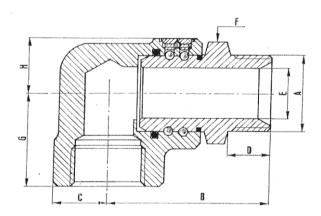
• Forged to ANSI B 16.11 Series 3000 in ASTM A105
